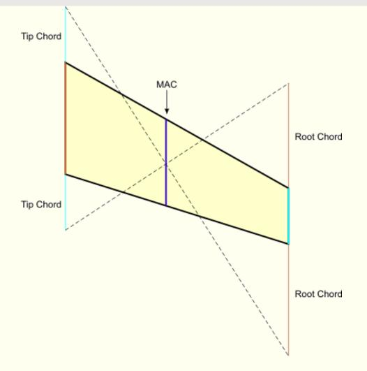
**Note:** The lines cross at the spanwise location of the MAC. It is not the fore/aft CG location (unless the CG happens to be located at 50% MAC).
